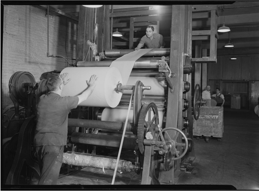
A SUPER-CALENDER IN A HOLYOKE PAPER MILL, 1936-37
